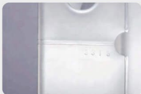
Material Traceability Identify and trace the steel material
